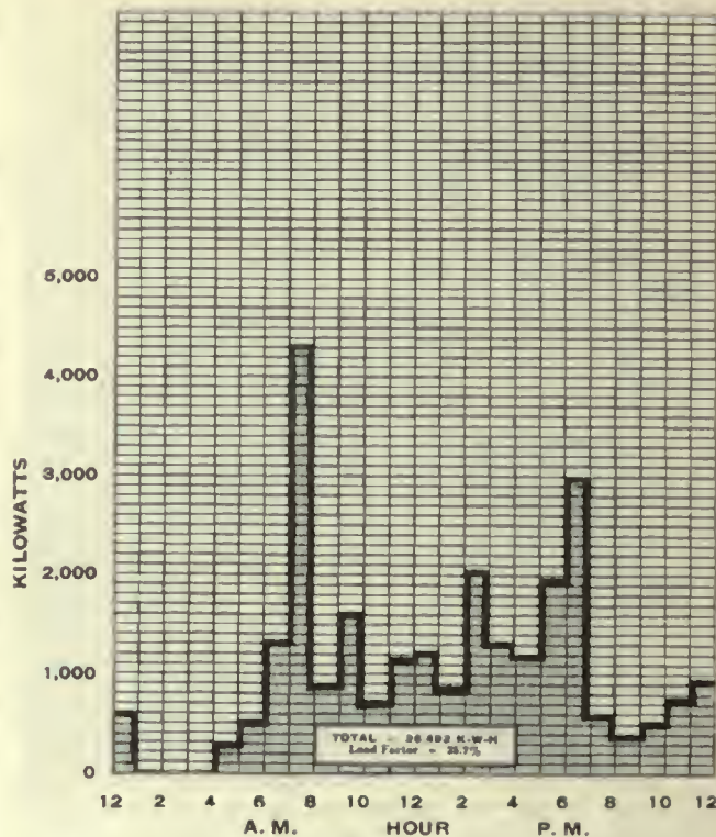
FIG. 618. ENERGY CHART. Kilowatt-Hours at the Pantograph for the Average October Day for 2,400-Volt D. C. Operation, Suburban Passenger Service with Locomotives on the C. & N. W. Ry.
